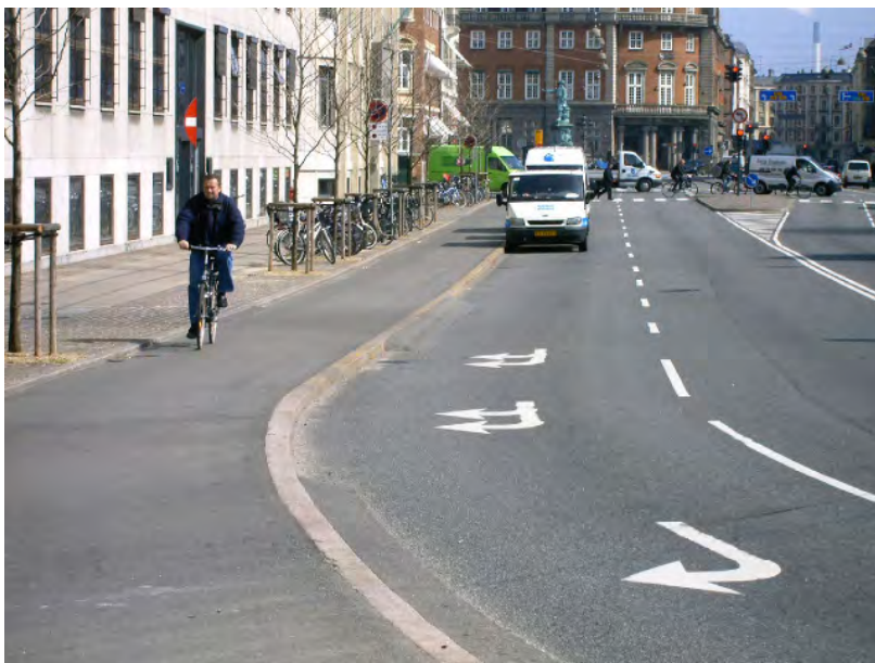
Figure 5-5: Raised Cycle Track 17
